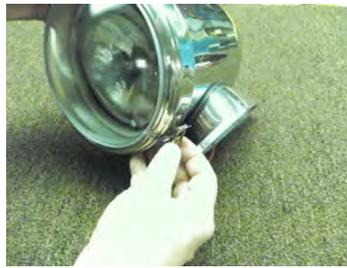
**STEP 2:** Using a 1/2” socket wrench or nut driver, remove the two hex bolts underneath the pedestal. Separate the bullet enclosure from the light housing assembly.
