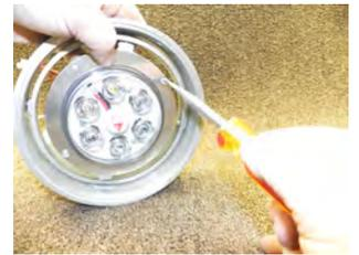
**STEP 7: LED Driver Hook-up:** Attach the black wire with ring terminal to the blackplate using one small nut and bolt that were removed in step 4. This is the ground screw for the LED driver.
