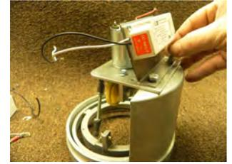
**STEP 6:** Position the LED module onto the front face of the unit. The wires should exit the module. Be sure the module is rotated so that the black and red wires are at the 2 o'clock position. Proceed to reinstall and tighten the two screws in the front face of the LED module.
